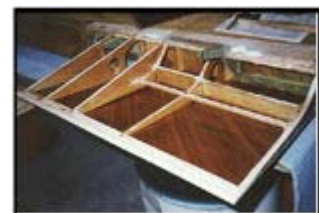
New ribs fabricated and installed
